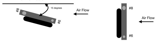
Looking at the end of the condenser, the small port should always be lower than the large port.
