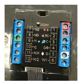
R- #1 Red 24VDC +in from a/c control board / thermostat power
